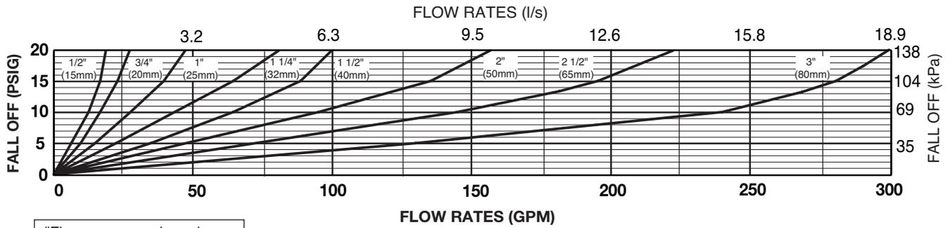
"Flow curves are based on a 50 psi pressure differential"
