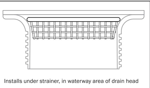
Installs under strainer, in waterway area of drain head
