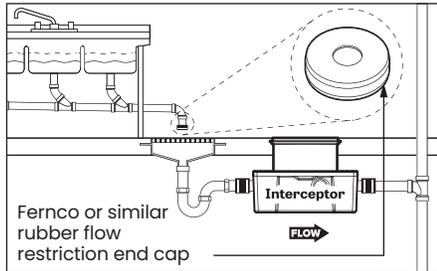
See drawing for guidance. For detailed guidance on indirect connections, go to: [webtools.schierproducts.com/Technical\\_Data/Indirect\\_Connections.pdf](http://webtools.schierproducts.com/Technical_Data/Indirect_Connections.pdf)
