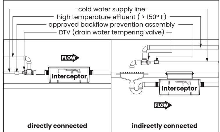
If water is entering the interceptor at excessive temperature (over 150° F), a drain water tempering valve (DTV) and approved backflow prevention assembly must be installed. Most state and local plumbing codes prohibit water above 150° F being discharged into the sanitary sewer. Water above 150° F will weaken or deform PVC Schedule 40 pipe, poly drainage fixtures like interceptors and erode the coating of cast iron (leading to eventual failure).
