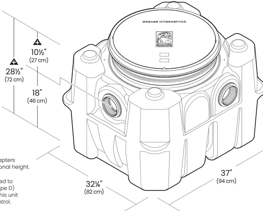
Adjustable cover adapters provide up to 4" of additional height.
