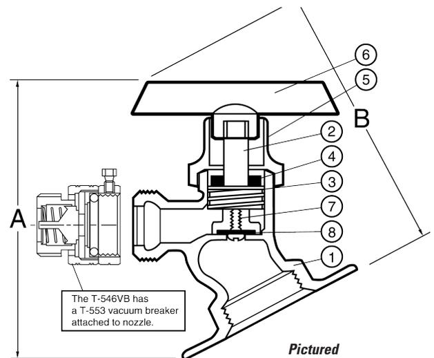
The T-546VB has a T-553 vacuum breaker attached to nozzle.
