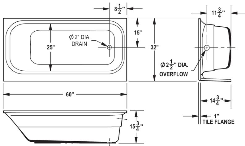
**General:** Furnish and install as shown on plans, TOPAZ® bathtub as manufactured by E.L. Mustee & Sons, Inc. Shall be a fiberglass 32" x 60": right hand or left hand Model \_\_\_\_\_. Construction shall be molded, reinforced fiberglass using matched metal molds under extreme heat and pressure. Shall meet ANSI Specification Z 124-2017. Color: \_\_\_\_\_ (White) Weight: 55 lbs. Install in compliance with local codes.
