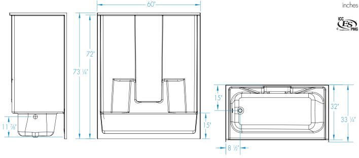
FEATURES 1bs Dimensional Tolerance ± %". Dimensions needed for site preparation should be measured from the unit. Aquatic assumes no responsibility for preparatory work.
